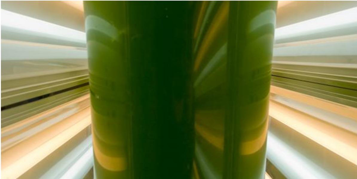
A bag of algae is hung between a row of lights at General Atomics facilities. Photo: Sam Hodgson
